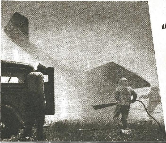
3—CO<sub>2</sub> is poured onto the fire as an ambulance stands by.
